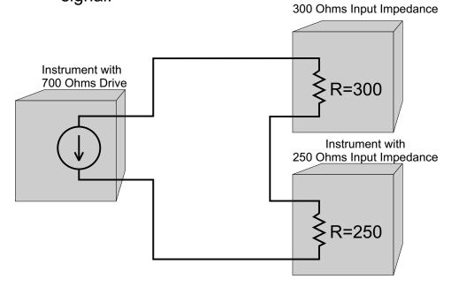
The total loop resistance in this loop is 300+250=550 ohms. The output drive of the left instrument is 700 ohms. This means that the output of the left instrument is almost loaded to capacity. No More instrument could be connected to this loop (except if its input impedance is less than or equal to 150 ohms).
