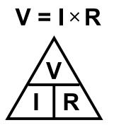
V=Voltage in Volts (V) I=Current in Amps (A) R=Resistance in Ohms (Ω) (also called Load)
