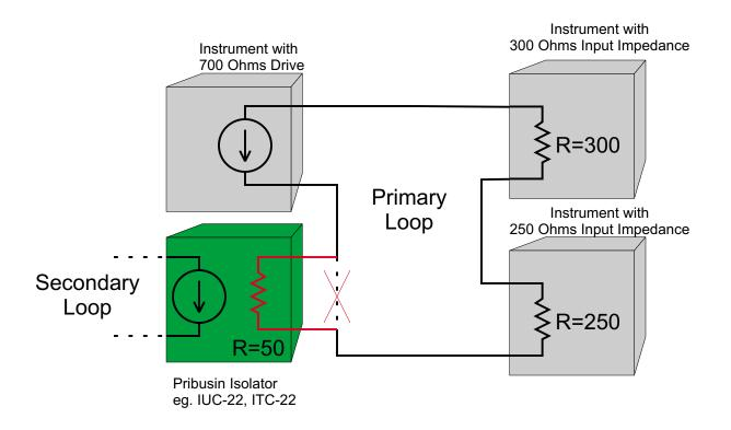
By adding a Pribusin Isolator into the Primary Loop the Primary Loop load increases by only 50 ohms to a total of 600 ohms. This is still well within the drive capability of the Primary Instrument.
