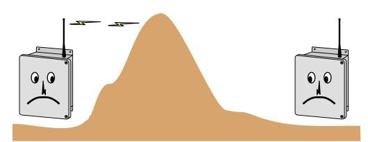
If there is a large physical obstruction between the two antennas, the radio waves will be blocked. No transmission is possible in this case.
