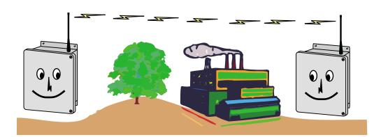
In the ideal system setup, both antennas can 'see' each other without any obstructions. This yields the greatest transmission distance and the most reliable signal conditions. This is called line-of-sight transmission.
