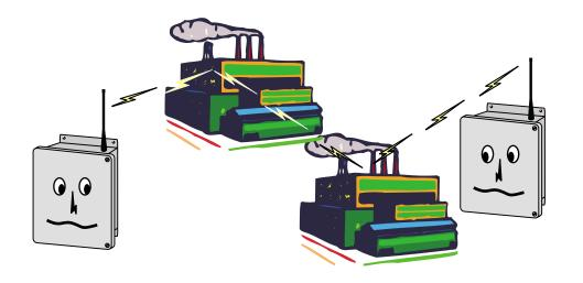
In many cases where there is no direct line-of-sight path between antennas, the RF signal may still get through by 'bouncing' off buildings or other solid structures. Signal strength must be taken into consideration here to determine if there is enough signal available for reliable transmission.
